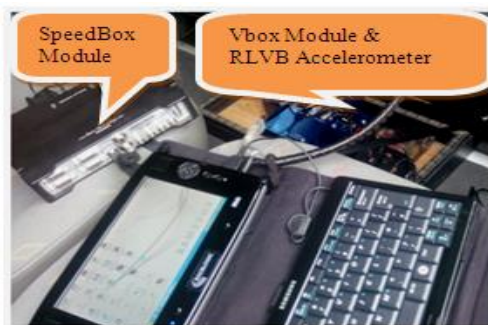
Figure 8. Installing SpeedBox and Vbox units Figure 9. Triaxial accelerometer RLVBIMU 03
