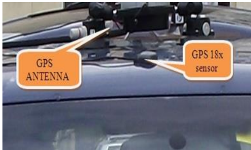
Figure 6. Mounting RF - GPS antenna on vehicle [2] Figure 7. Tracking system during travel [2]
