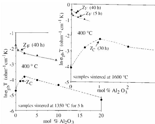
Fig. 6. Influence of the amount of alumina on  $\sigma_{gb}$  of samples  $Z_C$  and  $Z_F$
