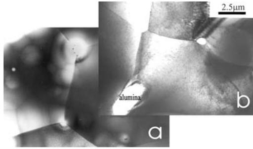
Fig. 3. Grain boundary microstructure of the Z<sub>F</sub> sample (a) sintered at 1600 °C, for 40 h, and of the Z<sub>F</sub> composite (b) sintered at 1350 °C, for 5 h.
