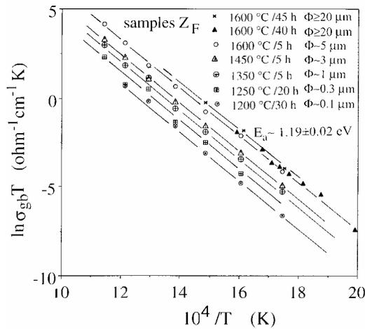
Fig. 4. Influence of the grain size on the grain boundary conductivity of samples Z<sub>F</sub>
