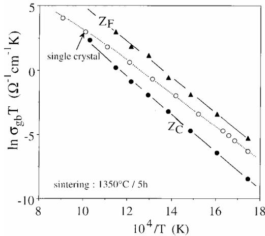
Fig. 5. Grain boundary conductivities of samples Z<sub>C</sub> and Z<sub>F</sub>. Comparison with the bulk conductivity of a single crystal (YSZ - 9 mol% Y<sub>2</sub>O<sub>3</sub>)
