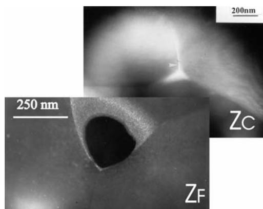
**Fig. 2. Grain boundary microstructure of the  $Z_F$  and  $Z_C$  samples.**
