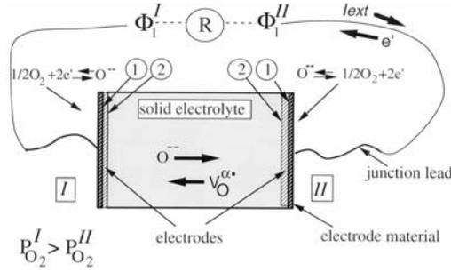
**Fig. 1. Experimental arrangement for electrochemical measurements ( $E_{open}$ ,  $t_{ion}$ ,  $D_O$ )**
