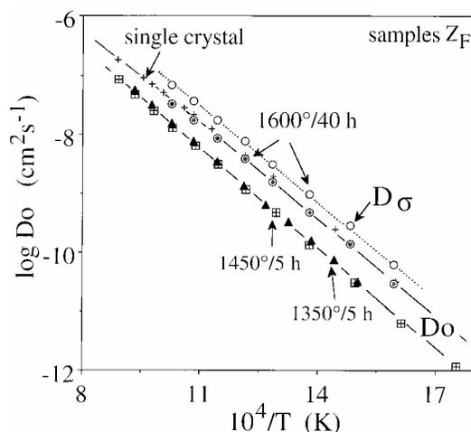
**Fig. 7. Oxygen diffusion coefficient of sample  $Z_F$  sintered at 1600 °C for 40 h. Comparison with the values obtained with a single crystal [7] and with those of  $D\sigma$**
