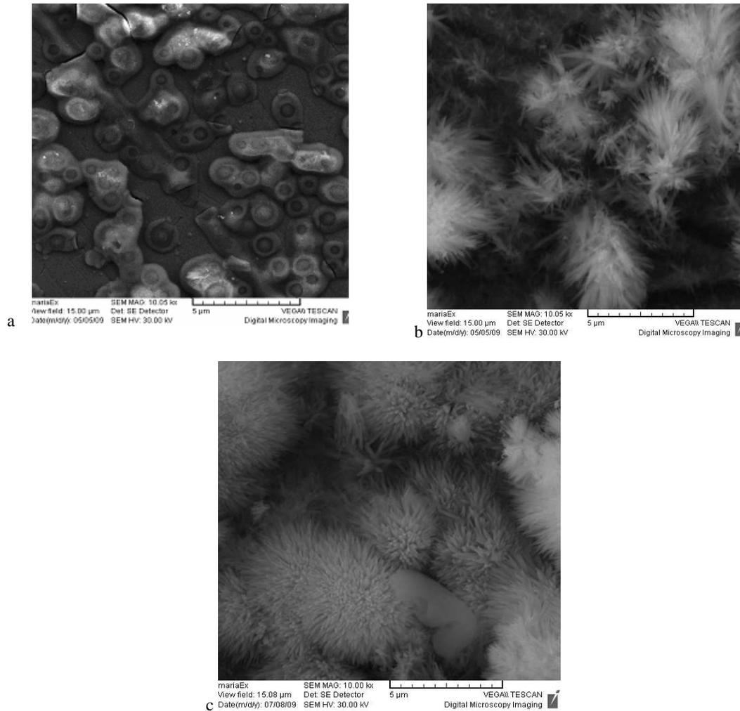
**Fig 3 SEM micrographs of the calcium phosphate deposited at -1,4V and 90 °C for various times: (a) 5 min, (b) 40 min, (c) 120 min.**
