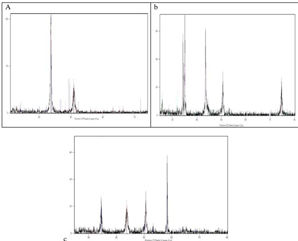
**Fig.5 Diagram X-ray diffraction of HAP coatings made on stainless steel 316L support: (a) 5 min, (b) 40 min, (c) 120 min**
