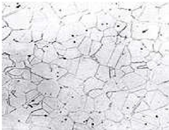
**Fig. 1 Microstructure of stainless steel 316L, 3% nital etching, 100X**
