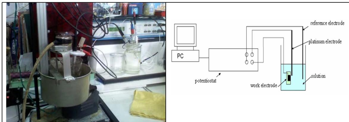
**Fig. 2 Electrochemical cell used for deposition**
