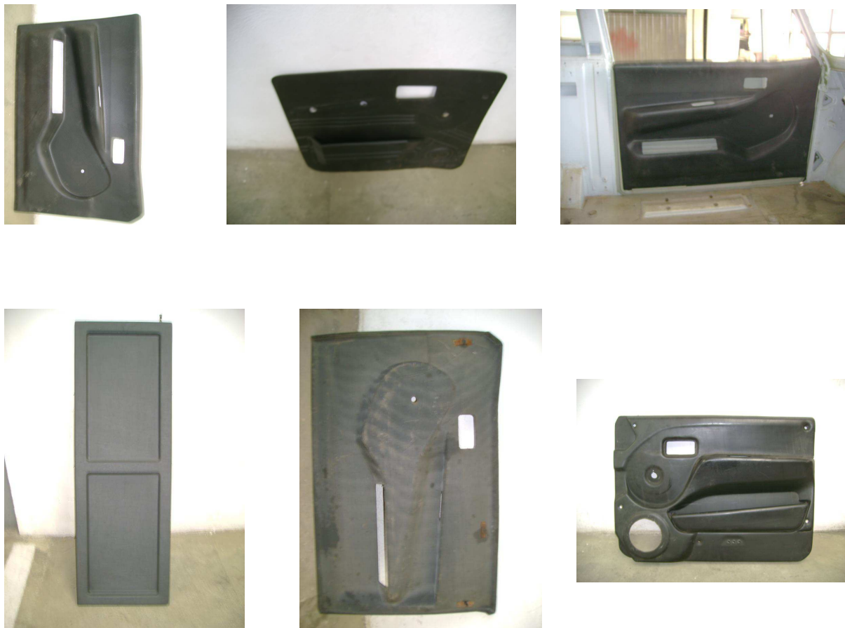
Fig.1. The parts obtained from the composite materials studied, used to fitted on the interior of the car.
