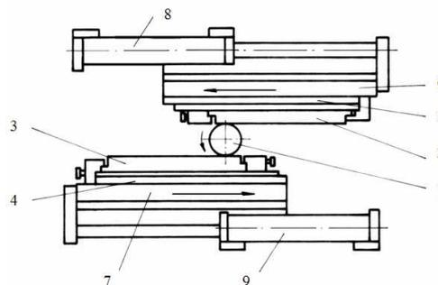
Fig. 2 Kinematical scheme of running the tool rack
