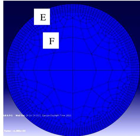
**Fig. 11 Discretization of the semi-product on radial direction**
