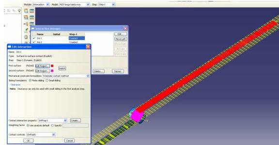
**Fig. “Surface to surface” type of contact**
