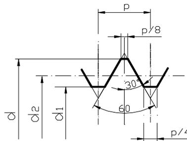
Fig.1 The form of the metric profile
