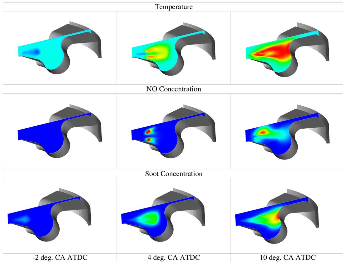
**Fig. 3. Temperature, NO and soot distribution at three different crank-angle positions [5]**
