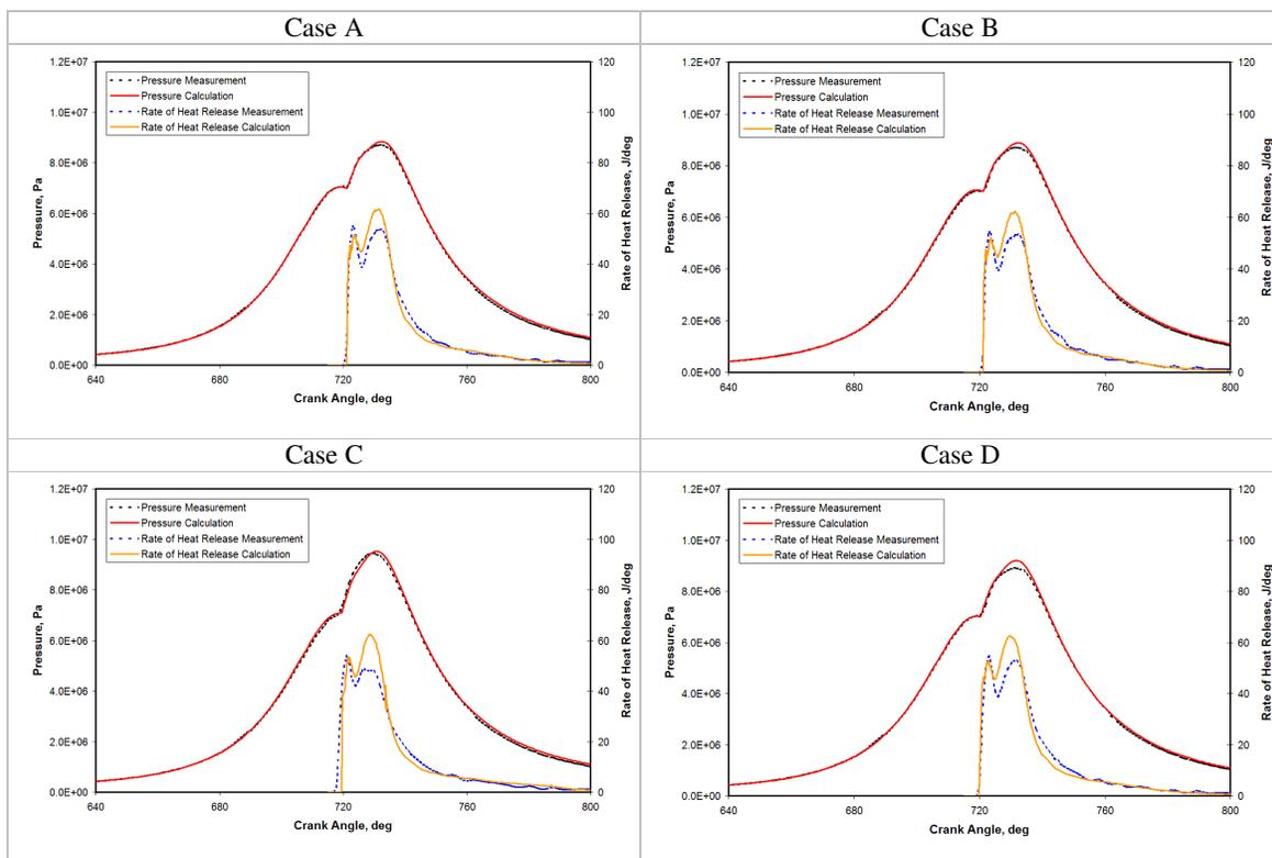
**Fig. 4. Calculated and measured pressure trace and rate of heat release for selected combustion system parameter variations [19]**
