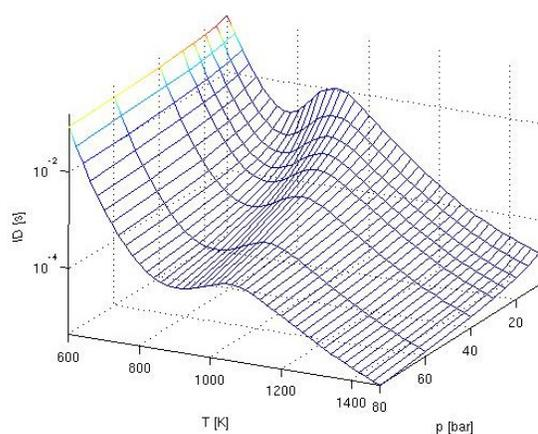
**Fig. 1. Tabulated ignition delay time as a function of temperature and pressure**
