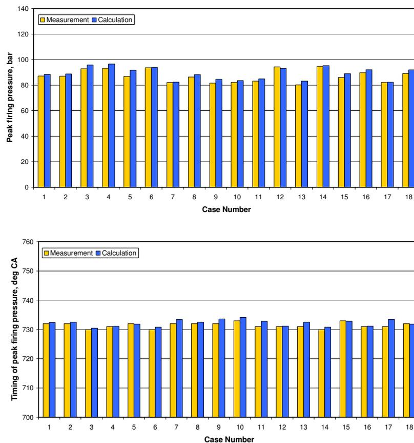
**Fig. 5. Comparison of calculated and measured peak firing pressure (top) and timing of peak firing pressure (bottom) for the investigated range of combustion system parameter variations [19]**
