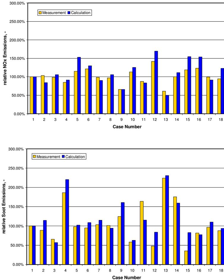
**Fig. 6. Comparison of calculated and measured normalized NO (top) and soot (bottom) concentrations for the investigated range of combustion system parameter variations**
