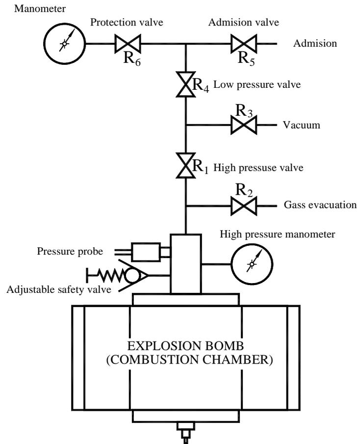
**Fig. 2. Hydraulic scheme of the explosion bomb.**
