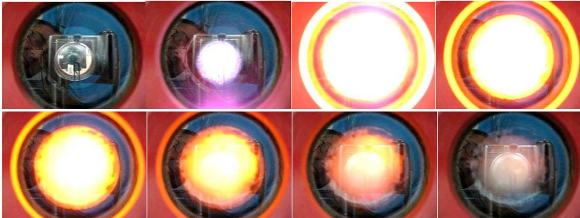
Fig. 5. Frames from the recording using classical ignition.
