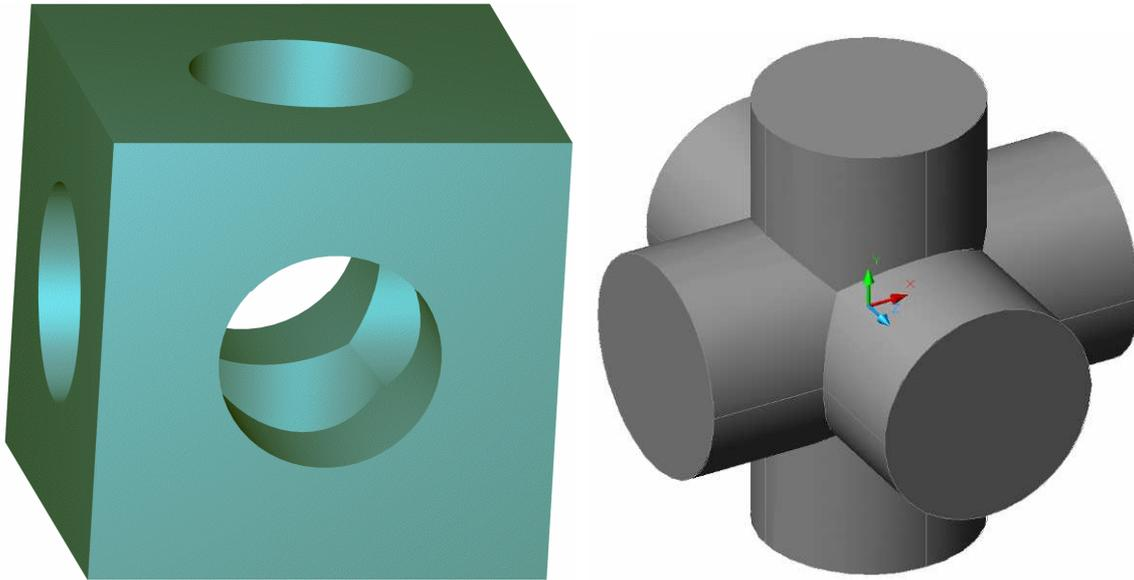
**Fig. 1. Spatial representation of the exterior and interior of the explosion bomb.**
