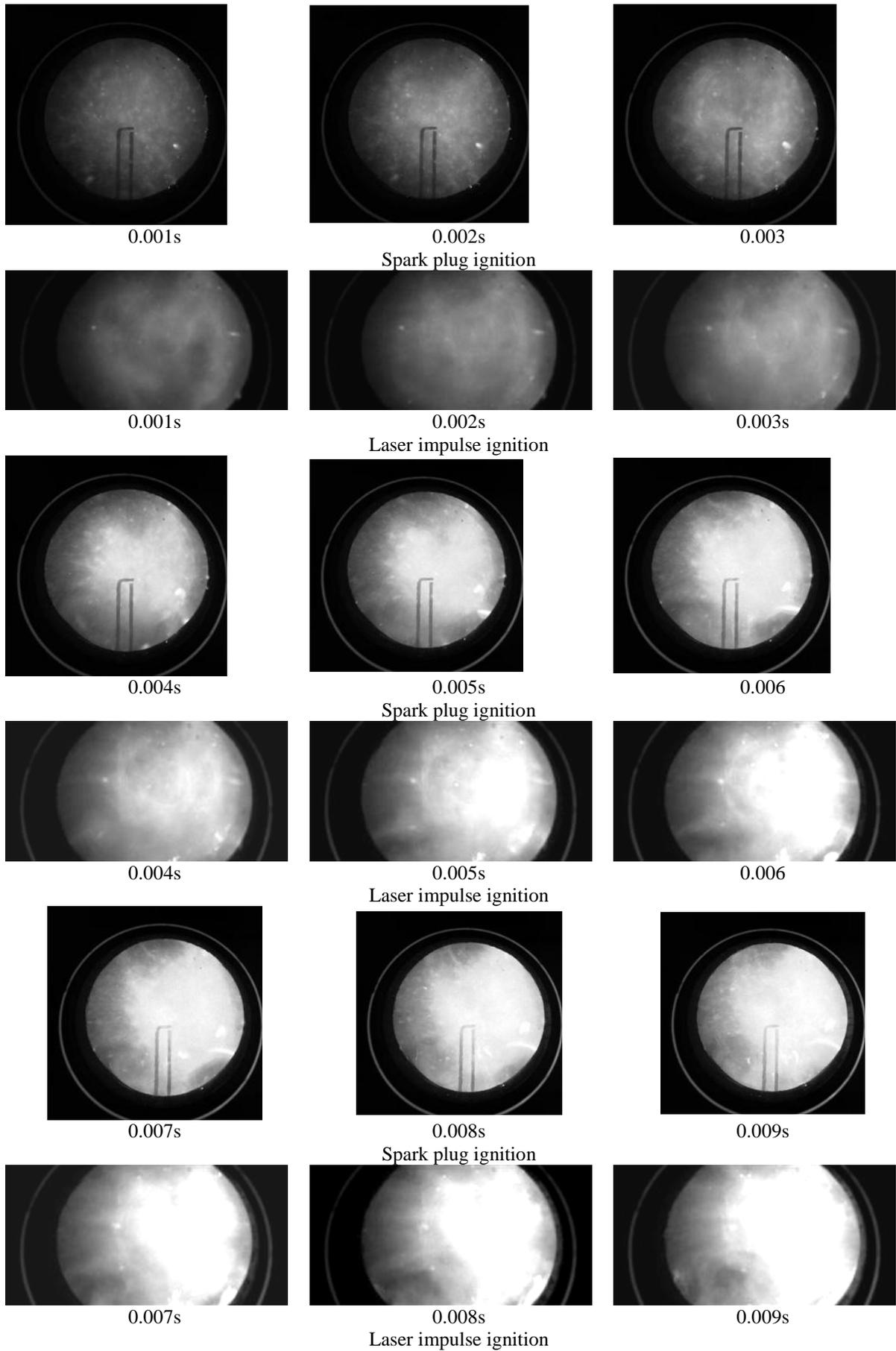
**Fig. 7. Frames from the recordings done with the rapid camera.**
