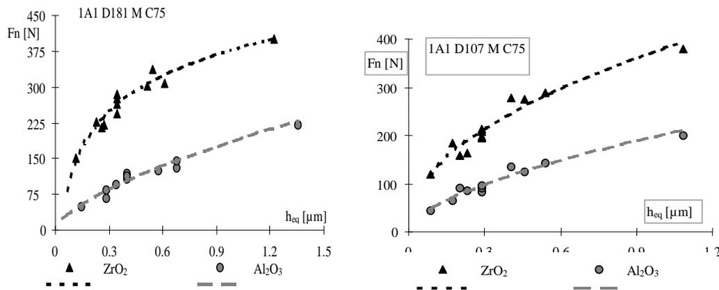
Figure 3 The variation of the conventional constituent of the cutting force function of the  $h_{eq}$
