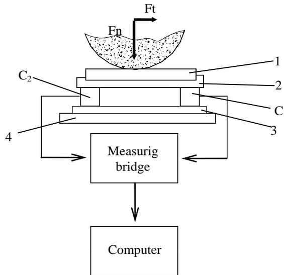
Figure 1. Block-diagram of the mounting used for measuring the grinding force constituents
