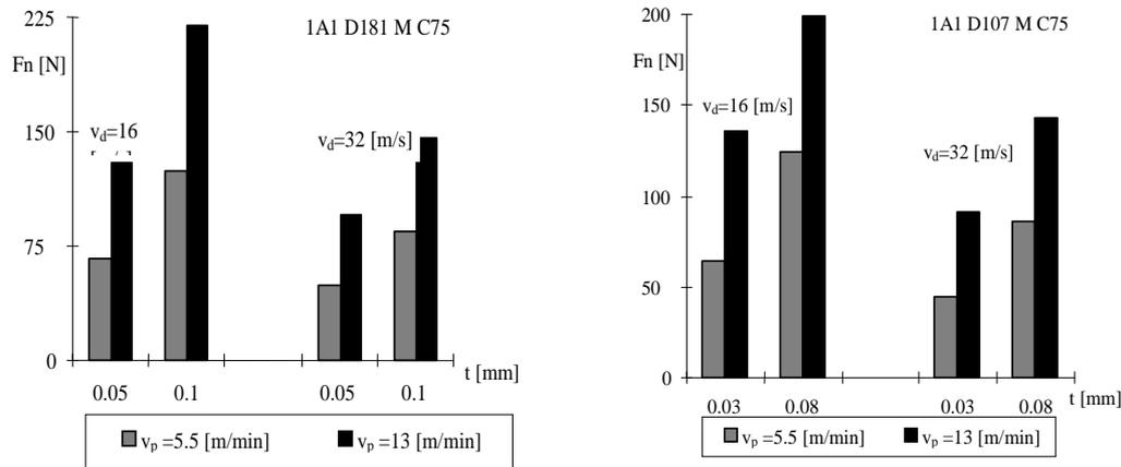
Figure 5. Dependency of the conventional constituent values of the cutting force to the grinding conditions parameters ( $v_d$ ,  $v_p$  and  $t$ ), in the  $Al_2O_3$  processing
