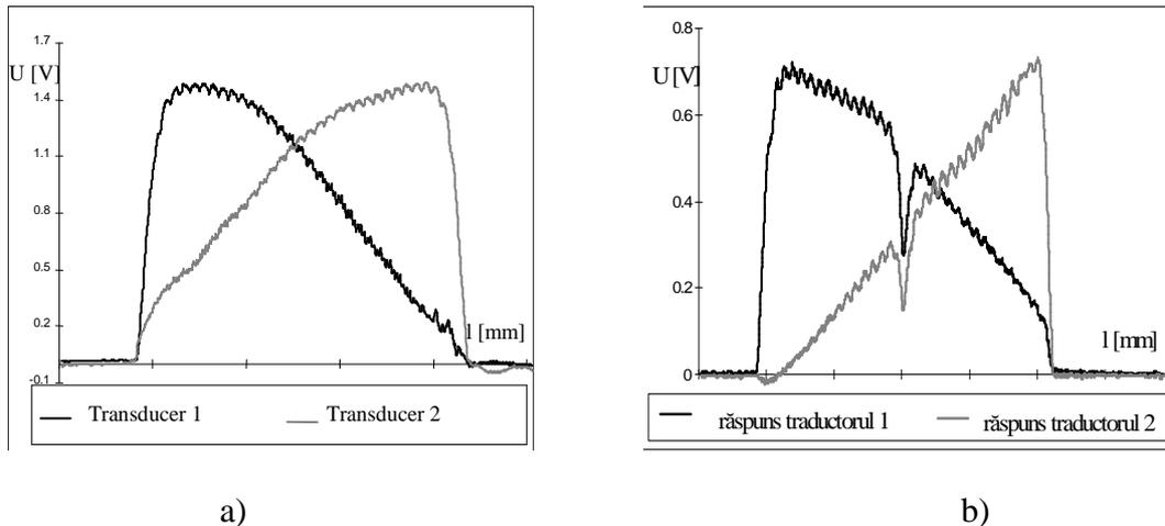
Figure 2. Variation of the signal given by the resistive transducers during processing
