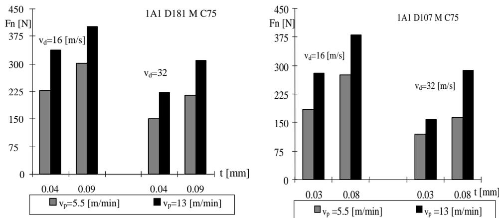
Figure 4. Dependency of the conventional constituent values of the cutting force to the grinding conditions ( $v_d$ ,  $v_p$  and  $t$ ), in  $ZrO_2$  processing
