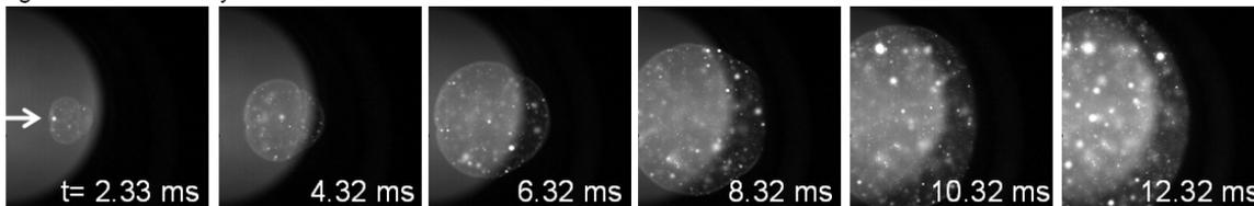
Figure 3. The evolution photographs of the spark plug and laser induced ignition with the conditions: methane-air mixture 12%, initial pressure of 0.1 MPa, the laser pulse energy of 22.8 Mj; the arrow shows the propagation in the case of laser induced ignition.
