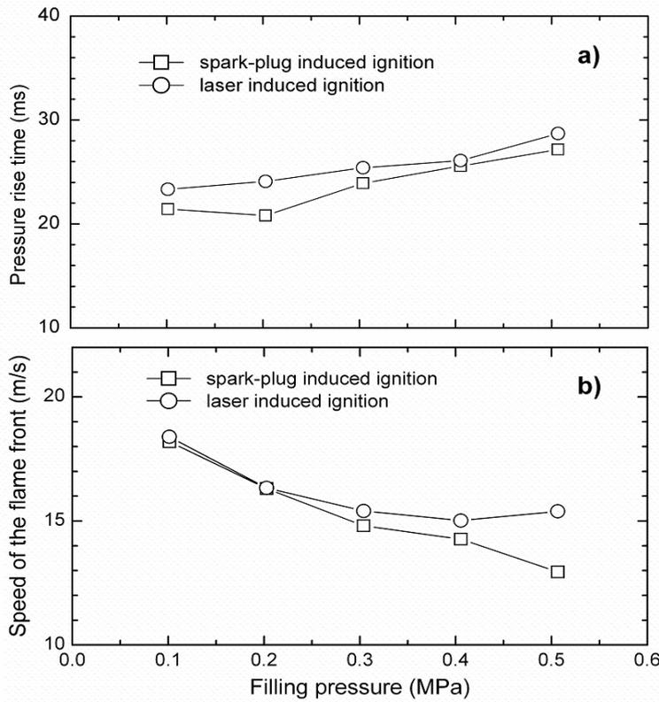
a) The time that the pressure developed by the explosion increases from 10% of the peak level to the maximum value.
