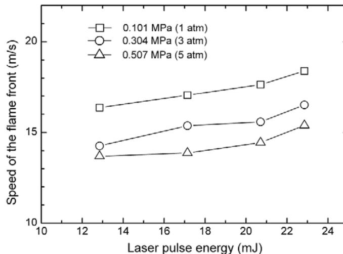
Figure 7. The velocity of the flame front propagation depending on the initial pressure in the combustion chamber and the energy of the laser pulse.
