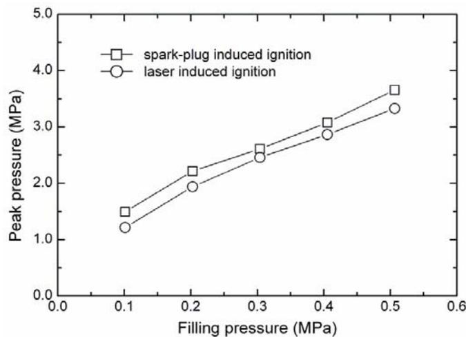
Figure 5. Peak developed pressure depending on the initial pressure in the explosion chamber.
