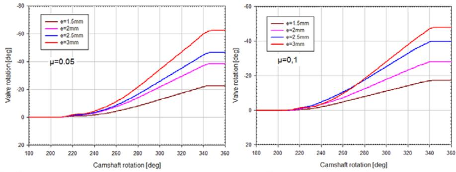
**Figure 7.** Comparison between valves rotation for different values of the cam eccentricity and different friction coefficients [3600rpm camshaft speed]
