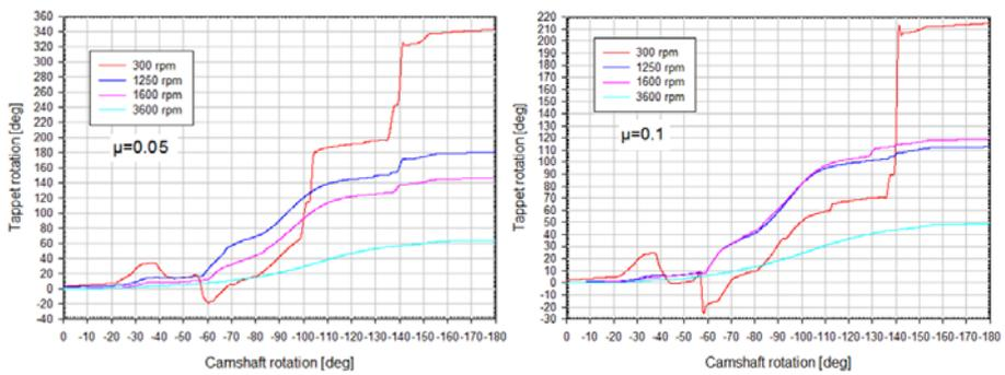
**Figure 9.** Comparison between tappets rotation for different friction coefficients and different camshaft speeds [2.5mm cam eccentricity]
