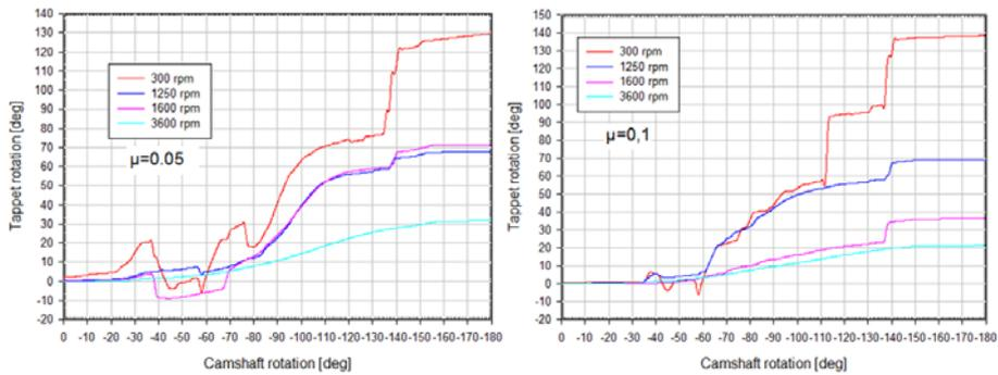
**Figure 8.** Comparison between tappets rotation for different friction coefficients and different camshaft speeds [1.5mm cam eccentricity]
