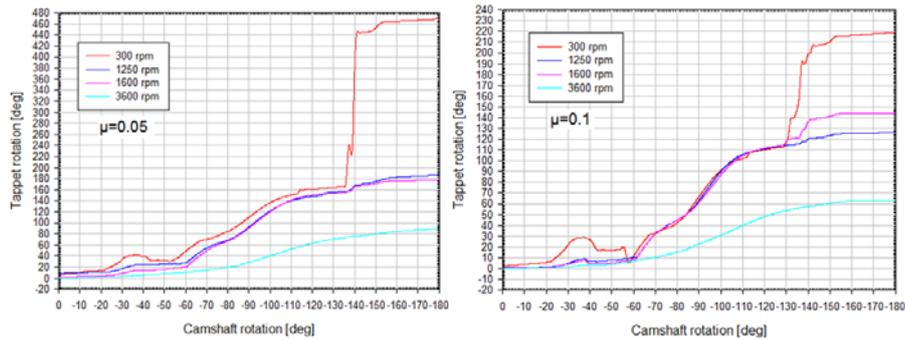
**Figure 10.** Comparison between tappets rotation for different friction coefficients and different camshaft speeds [3mm cam eccentricity]
