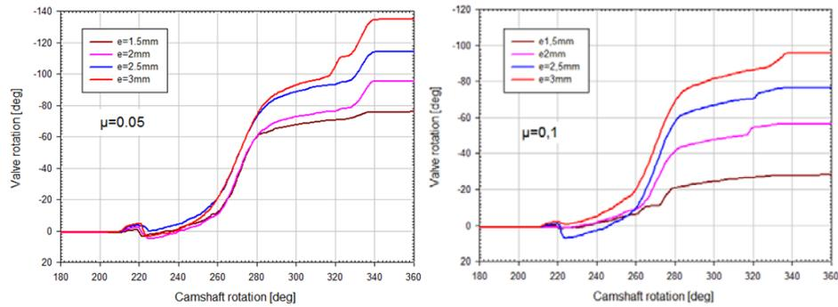
**Figure 4.** Comparison between valves rotation for different values of the cam eccentricity and different friction coefficients [300rpm camshaft speed]
