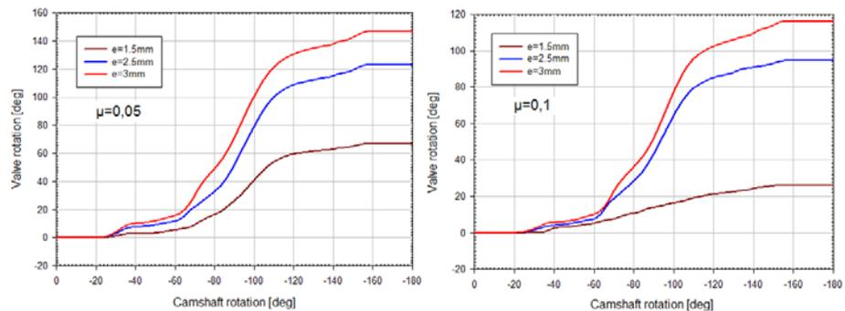
**Figure 6.** Comparison between valves rotation for different values of the cam eccentricity and different friction coefficients [1600rpm camshaft speed]
