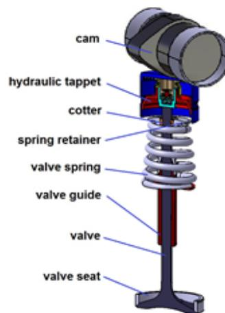
**Figure 1.** Components of the direct acting valve train system
