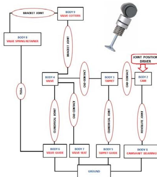
**Figure 3.** Design of the virtual model of the valve train
