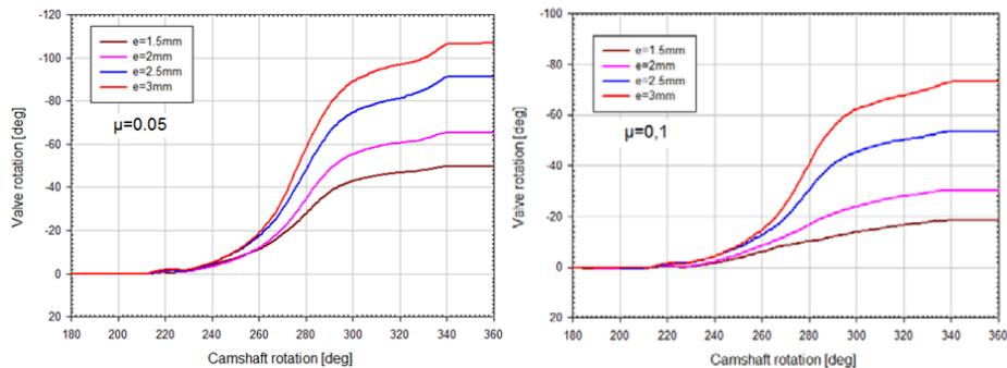
**Figure 5.** Comparison between valves rotation for different values of the cam eccentricity and different friction coefficients [1250rpm camshaft speed]
