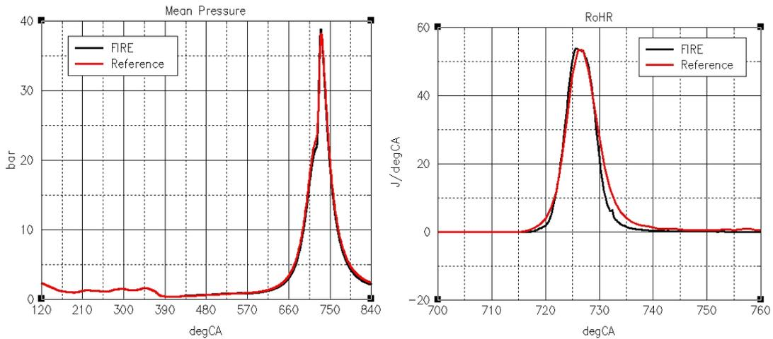
**Figure 10.** SCRE CAI – Pressure and Rate of Heat Release – 2000 rpm / 3 bar, E85
