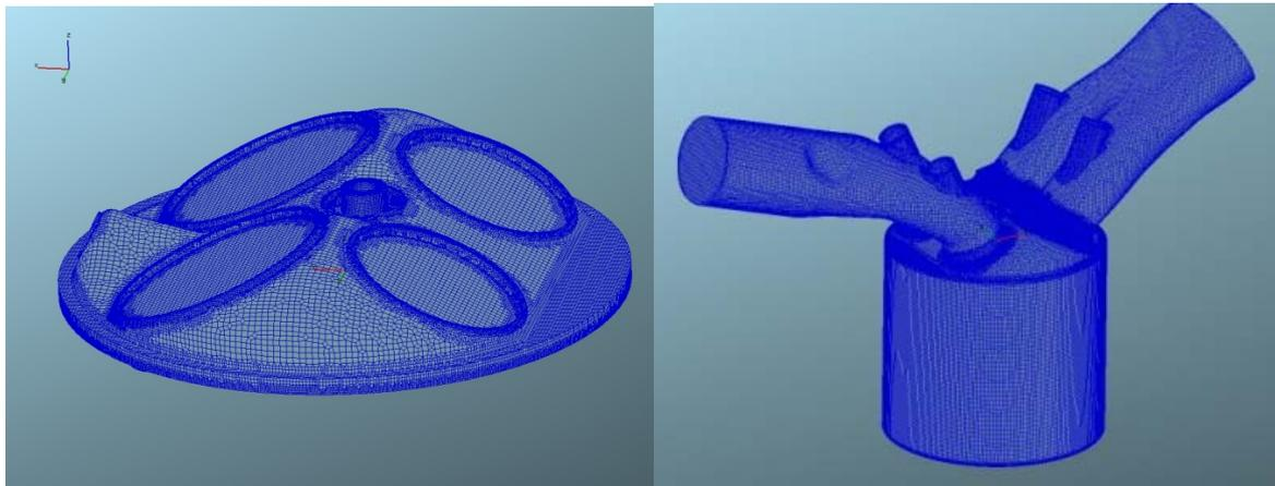
**Figure 7.** Mesh model of the SCRE Engine.
