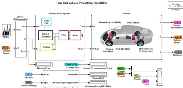
**Figure 3.** Global model in Simulink
