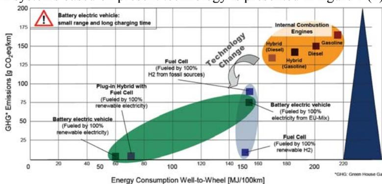
**Figure 1.** Energy consumption vs. green house gas emissions for different propulsion systems
