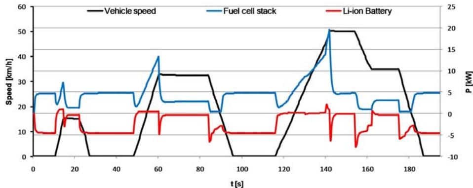
**Figure 12.** Vehicle speed and electrical power for fuel cell stack and battery during ECE15 cycle
