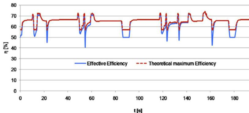
**Figure 13.** Fuel cell stack efficiency during ECE15 simulation
