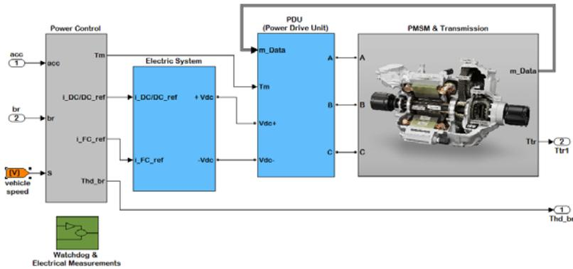
**Figure 4.** Electric Drive System
