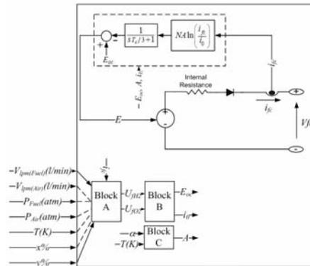
Figure 10. PEM Fuel Cell equivalent electrical circuit
