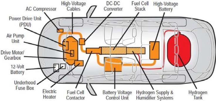
**Figure 2.** The main components of the powertrain of Honda FCX Clarity (2010 model)
