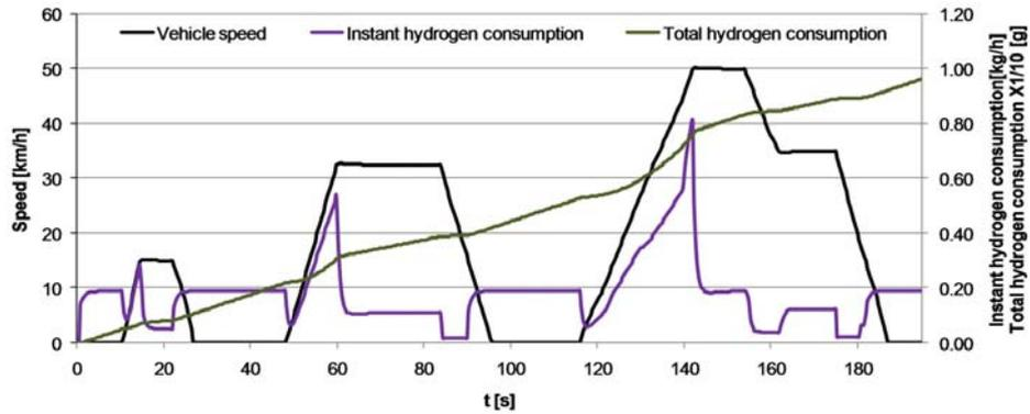
**Figure 11.** Hydrogen consumption and vehicle speed during ECE15 cycle
