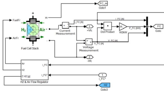
Figure 9. Fuel Cell Stack command and control
