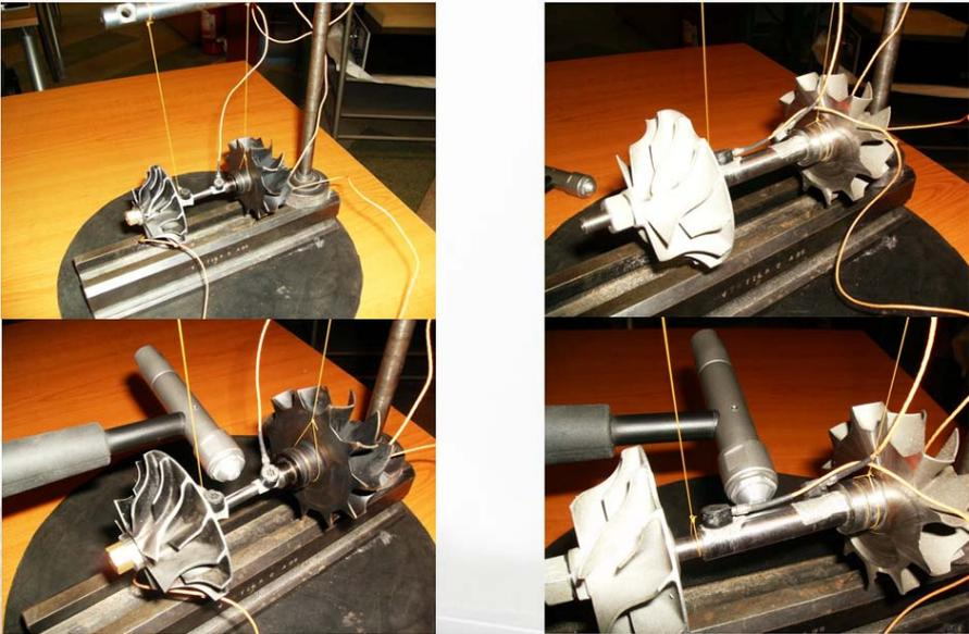
Figure 16. Accelerometer placement and hammer impact point
