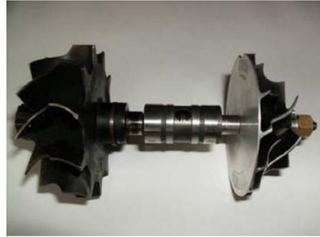
**Figure 2.** Modified turbocharger rotor
