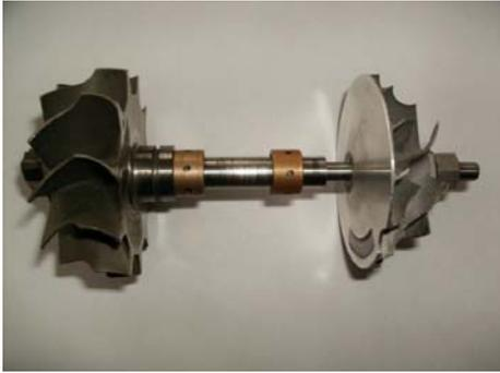
**Figure 1.** Classical turbocharger rotor
