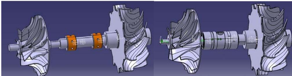
**Figure 3.** 3D model of classic rotor
