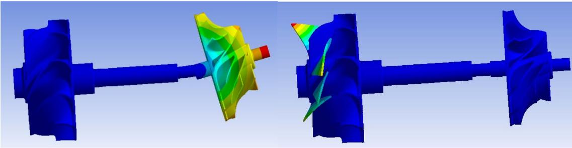
**Figure 5.** Mode shape for the classic rotor
