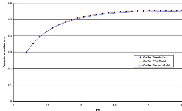
**Figure 6:** Reduced mass flow vs Pressure ratio plot: steady comparison of the models.
