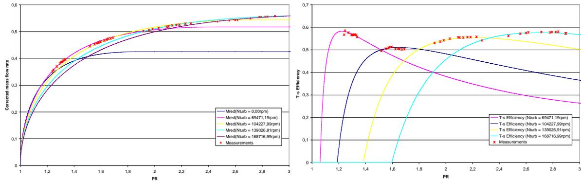
**Figure 5.** Results of the turbine data map extrapolations.
