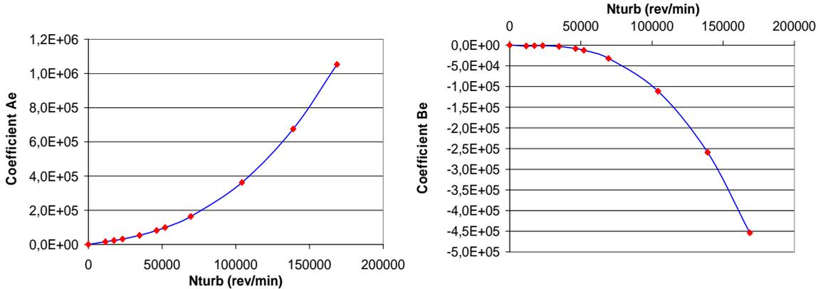
**Figure 4.** Evolution of the parameters Ae et Be, in function of the rotor velocity.
