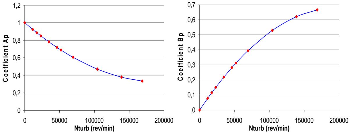
**Figure 3. Evolution of the parameters Ap et Bp, in function of the rotor velocity.**
