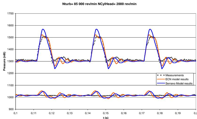
**Figure 8.** Comparison of measured and modelled inlet and outlet turbine pressures.
