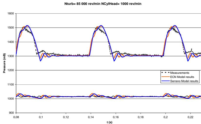
**Figure 7.** Comparison of measured and modeled inlet and outlet turbine pressures.
