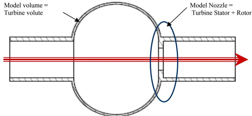
**Figure 1. Turbine model scheme.**
