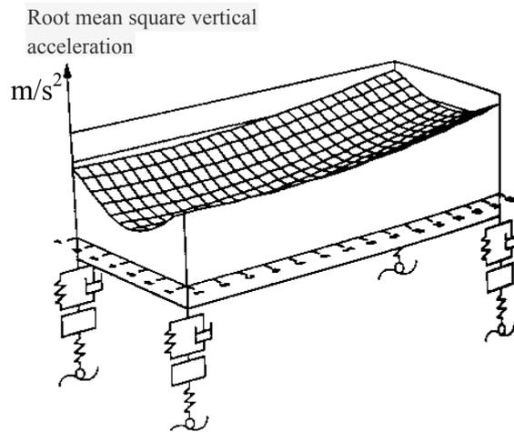
**Figure 8.** Values transmissibility function of vertical acceleration
