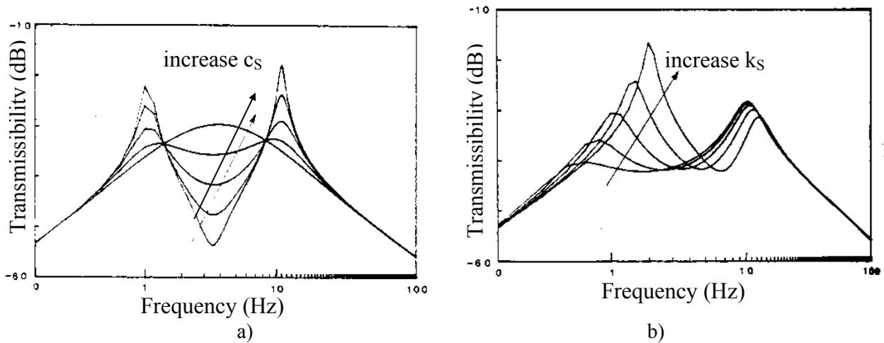
Figure 4. Transmissibility vs. frequency
