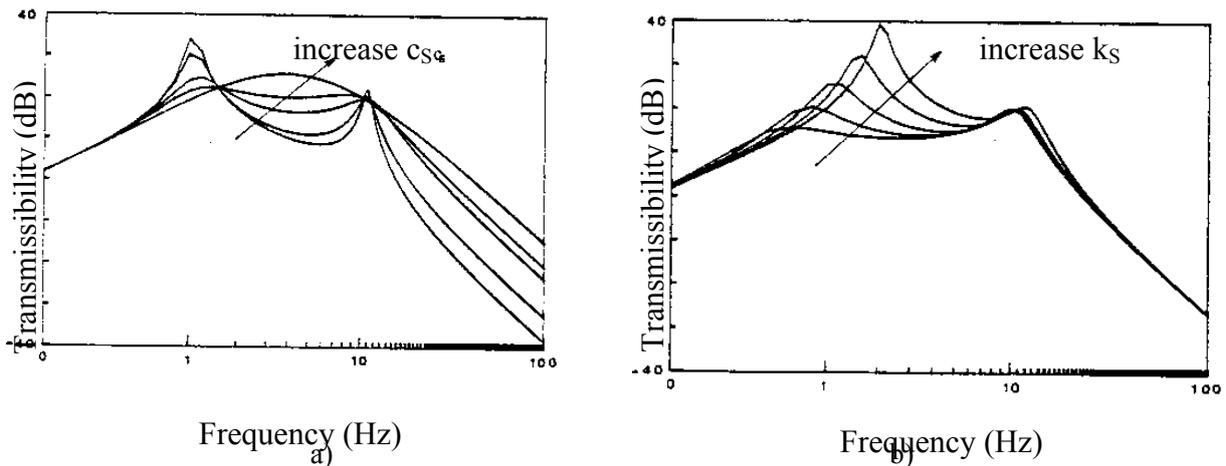
Figure 2. Transmissibility vs. frequency
