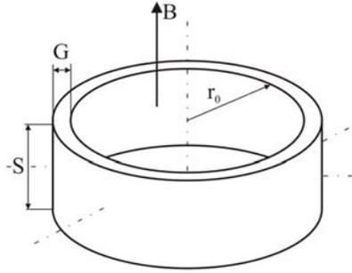
Figure 8. General shape of the rim section of a MRF in a MRF disc brake.
