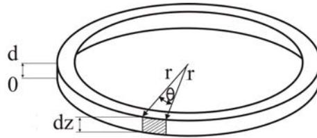
Figure 7. Approximation of the flank section of a MRF with emphasis on rim surface.
