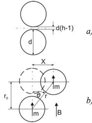
Figure 3. a) Geometry of two particles of diameter  $d$  within a particle chain, b) magnetic interaction of the two particles modeled as dipole moments  $|m|$  and sheared with respect to one another [18].
