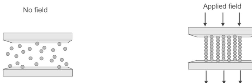
Figure 1. Chain-like structure formation in controllable fluids [4]
