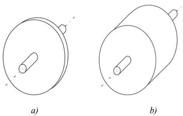
Figure 2. Two types of discs for MRF brake.
