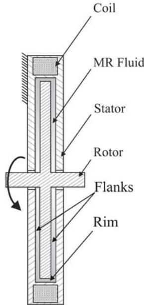
Figure 4. Main components of a MRF disc brake.
