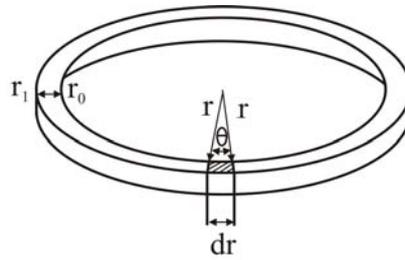
Figure 6. Approximation of the flank section of a MRF with emphasis on side surface.
