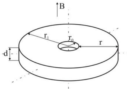
Figure 5. Simplified shape of the flank section of a MRF in a MRF disc brake.
