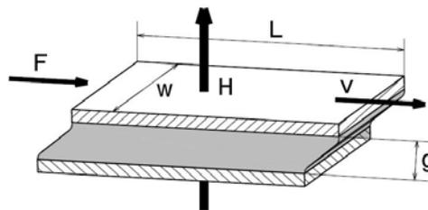
Figure 10. MRF in the shear mode [9]
