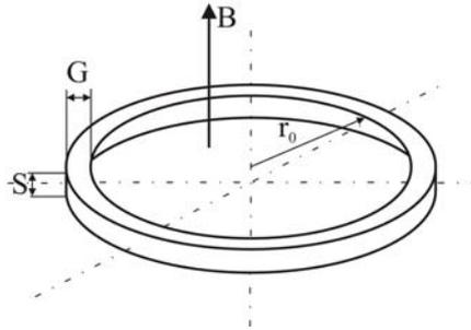
Figure 9. Thinner shape of rim section of a MRF in a MRF disc brake
