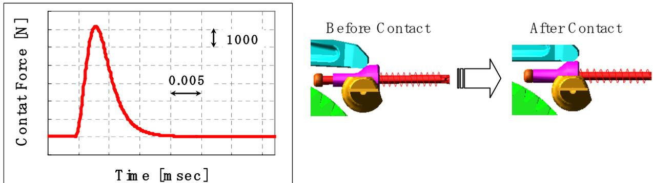
Fig. 3 Contact force between wedge and tube
