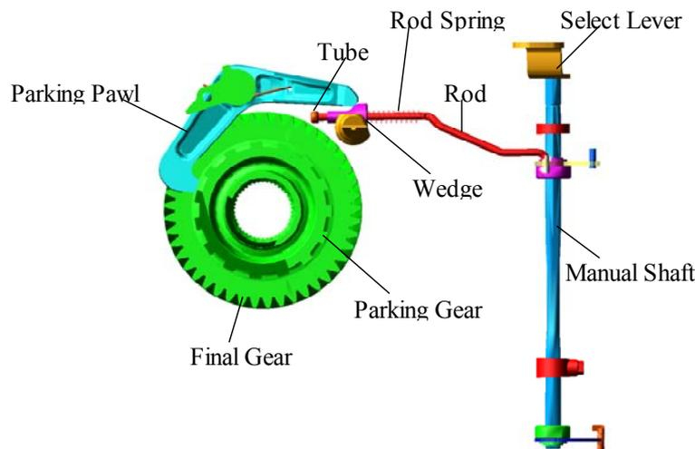
Fig. 2 Parts of parking system in AT
