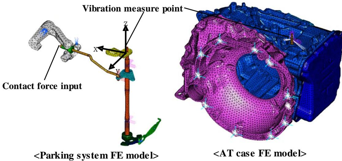
Figure. 4 FE model of parking system and case of AT
