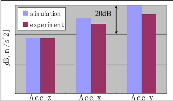
Figure.10 Vibrations at 10rpm of parking gear
