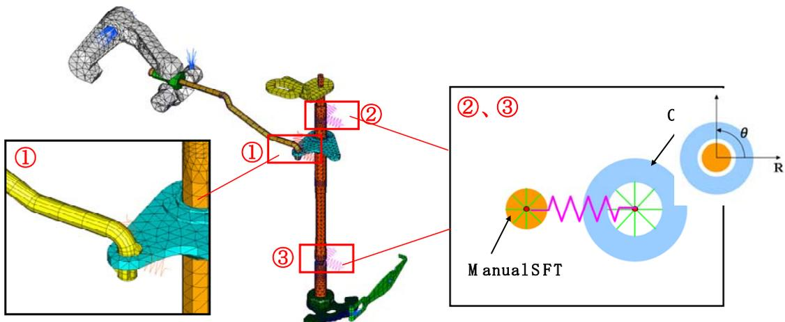
Figure 5. three main constraints affecting vibration
