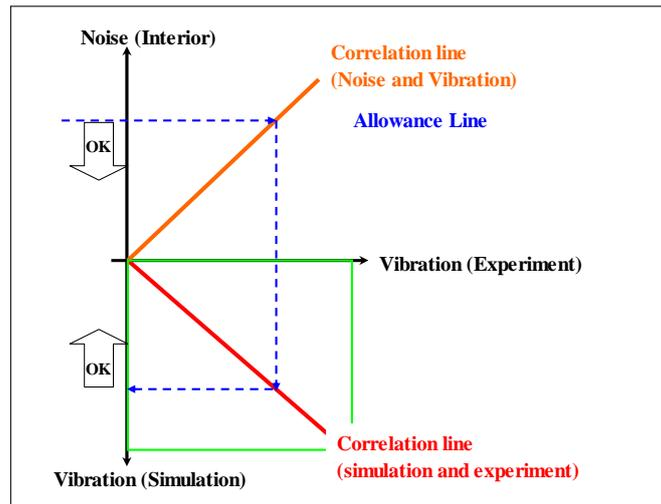
Figure. 1 Correlation line for prediction of interior noise
