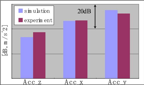
Figure.8 Vibrations at 3rpm of parking gear
