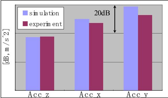
Figure.9 Vibrations at 6rpm of parking gear
