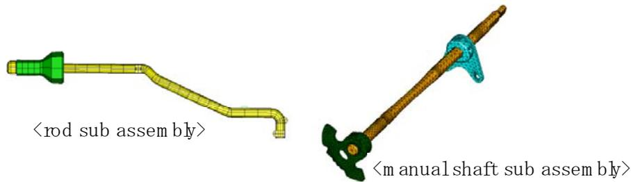
Figure 6. Rod and manual shaft sub assembly
