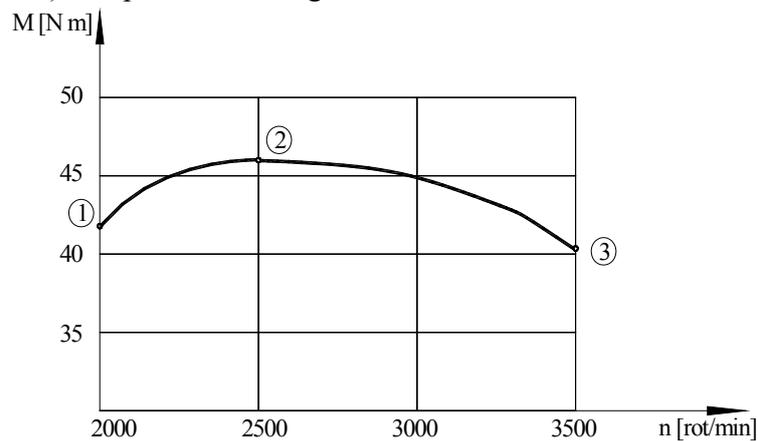
Fig. 7. The characteristic  $M(\omega)$  of the heat engine.
