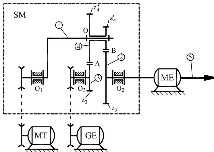
Fig. 1. The kinematic diagram of the mechanical system.
