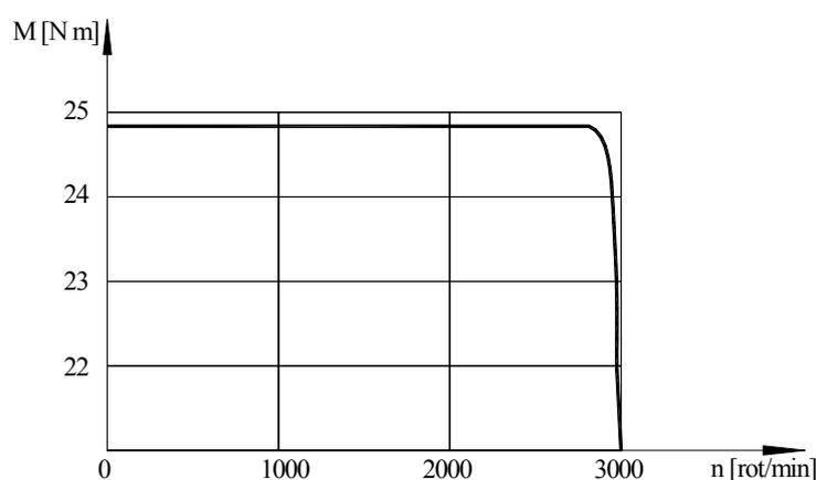
Fig. 8. The  $M(\omega)$  characteristic of the frequency controlled asynchronous engine.
