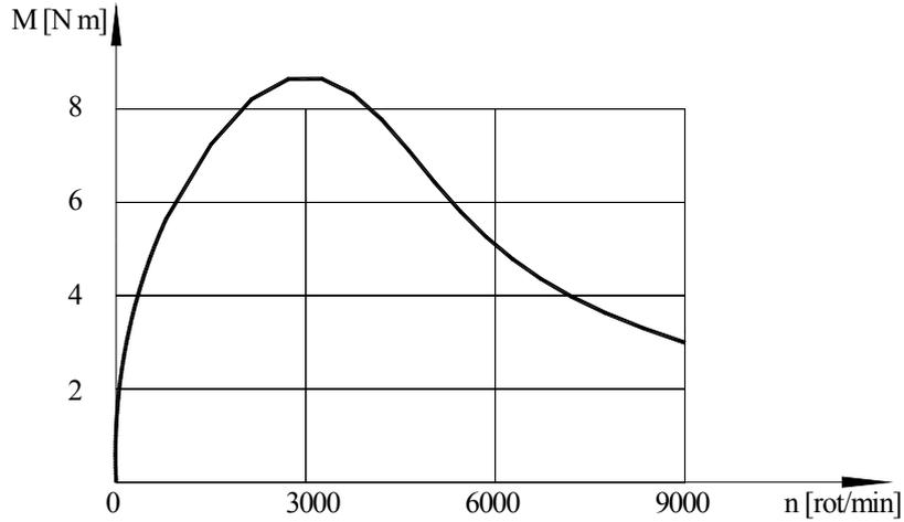
Fig. 9. The external characteristic of a 3 kW alternator.
