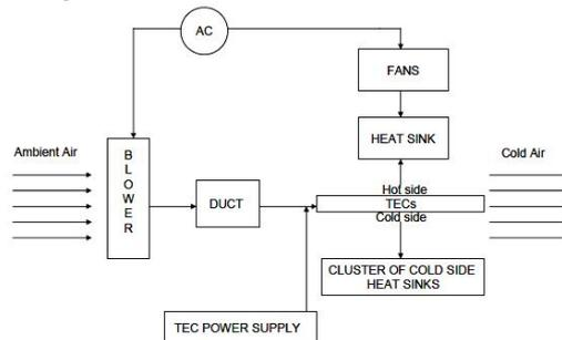
**Figure 5.** Block diagram of the thermoelectric cooled cooling fan.
