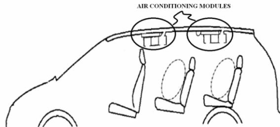
**Figure 7.** Schematic sectional view of a vehicle cabin equipped with two ventilating, heating and/or air conditioning modules.
