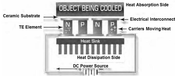
**Figure 1.** A Classic Thermoelectric Module Assembly
