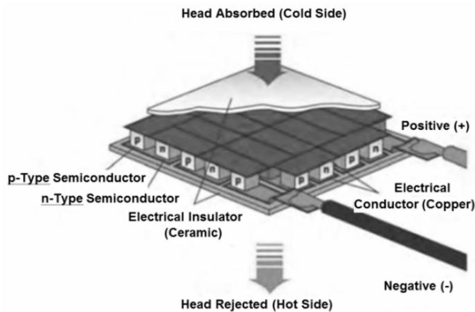
**Figure 2.** The Construction of a Thermoelectric Module
