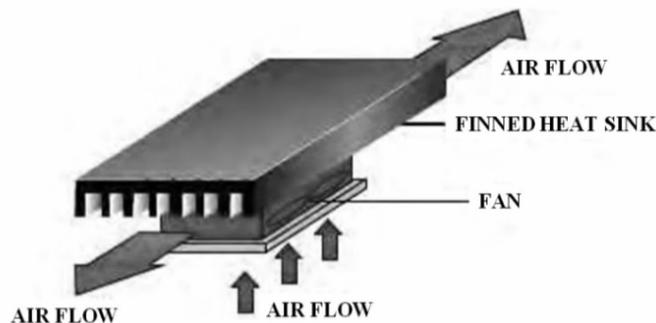
**Figure 4.** Forced convection heat sink system
