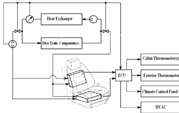
**Figure 9.** Schematic system diagram of a thermoelectric comfort control system
