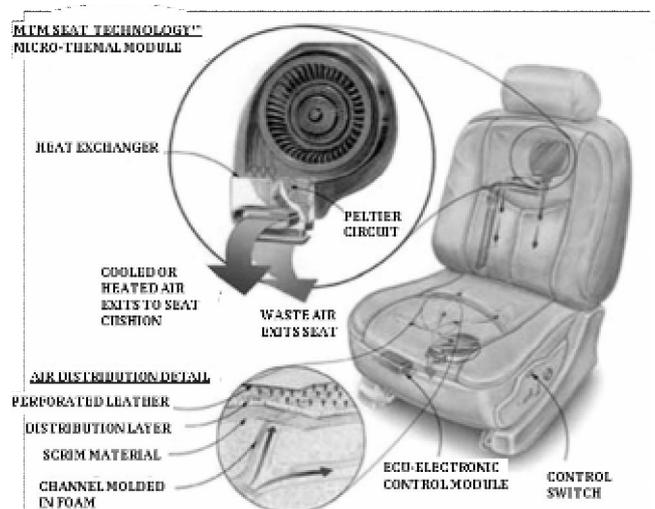
**Figure 8.** Amerigon’s Peltier module CCS system (Courtesy of Amerigon Corporation)
