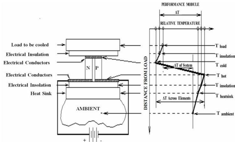
**Figure 3.** Characteristics temperature of relationship in a thermoelectric cooler
