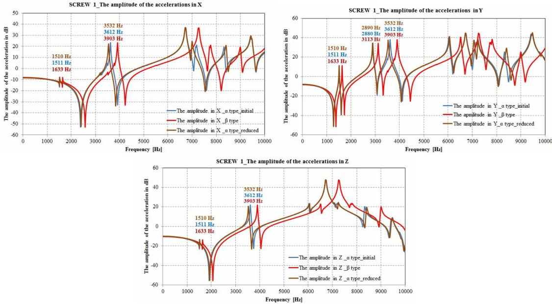
**Figure 6.** Comparative analysis of FRF for vented cast iron discs type  $\alpha/\beta/\text{type } \alpha$  reduced when effort is applied.
