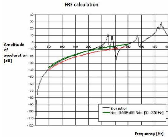
**Figure 5.** Graphic representation of a FRF curve.
