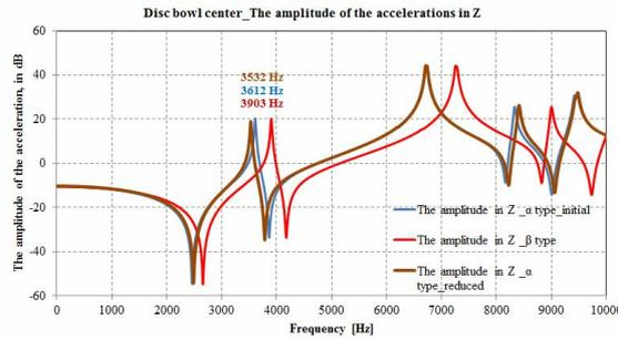
**Figure 10.** Comparative analysis of FRF for vented type  $\alpha/\beta$ /type  $\beta$  reduced cast iron disks, when effort is applied in the disk bowl center, in 3 directions (vehicle coordinates).
