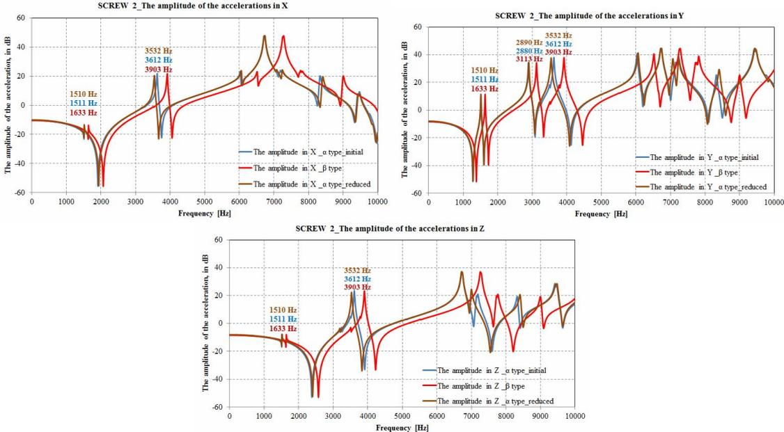
**Figure 7.** Comparative analysis of FRF for vented type  $\alpha/\beta/\text{type } \alpha$  reduced cast iron disks when effort is applied in fastening screw 2, on the 3 directions (vehicle coordinates).
