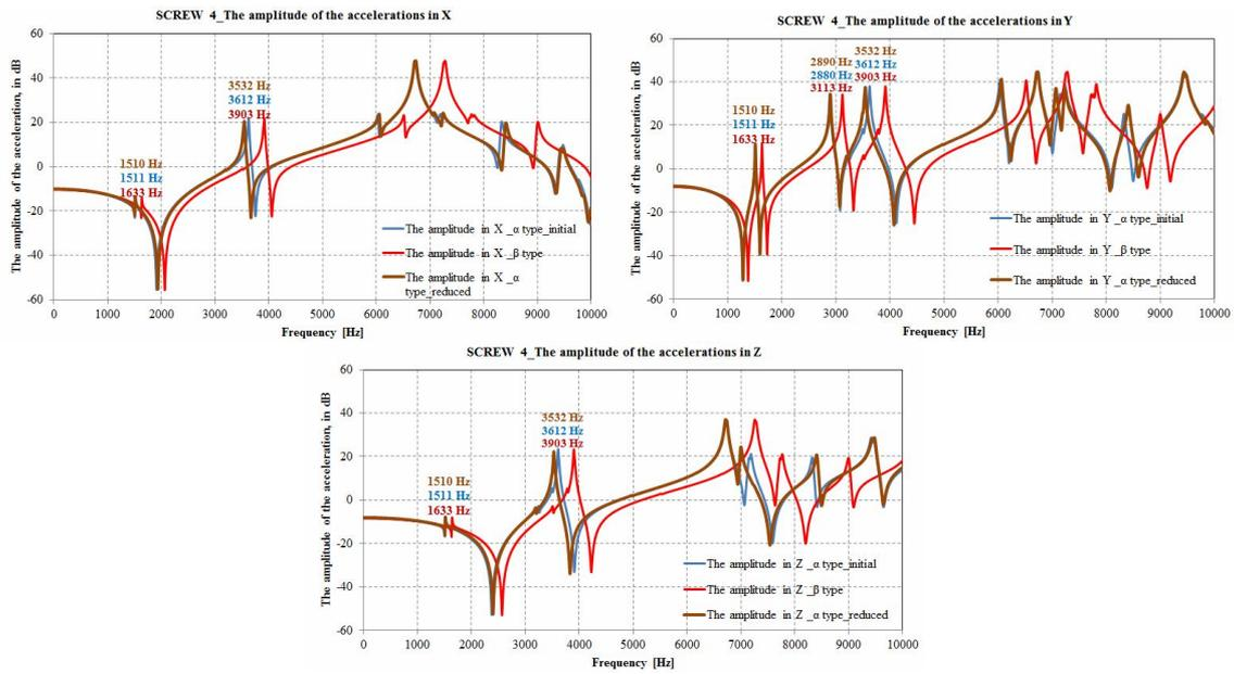
**Figure 9.** Comparative analysis of FRF for vented type  $\alpha/\beta$ /type  $\alpha$  reduced cast iron discs when effort is applied in fastening screw 4, on the 3 directions (vehicle coordinates).
