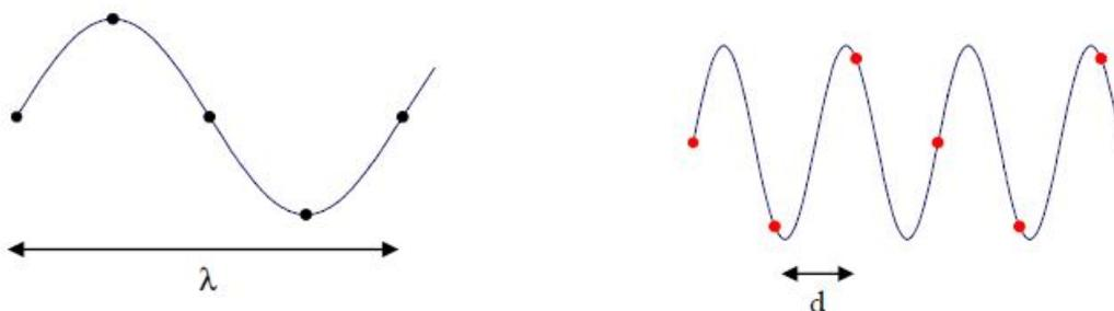
Long wavelength, which is the correct representation of deformation: four elements on a wavelength
