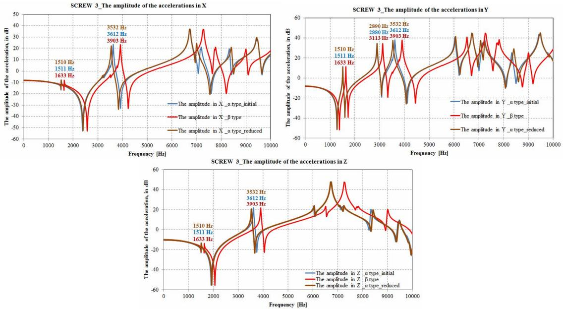
**Figure 8.** Comparative analysis of FRF for vented type  $\alpha/\beta$ /type  $\alpha$  reduced cast iron discs when effort is applied in fastening screw 3, on the 3 directions (vehicle coordinates).
