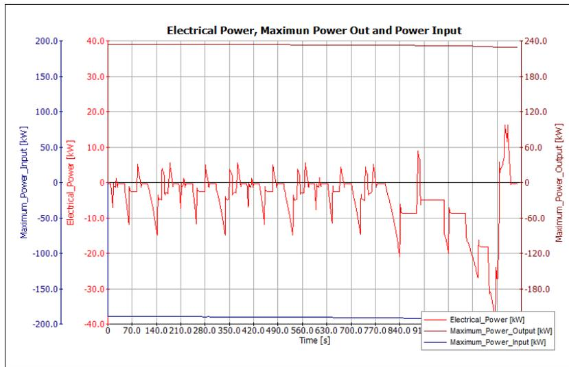
Figure 7. Electric power accumulated and consumed
