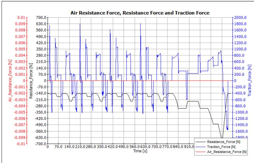
Figure 6. Variation air resistance, rolling resistance and traction in relation to time
