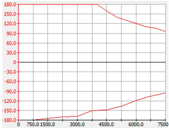
**Figure 2.** Torque characteristic in electric car accessories regime (top) and a generator (below)
