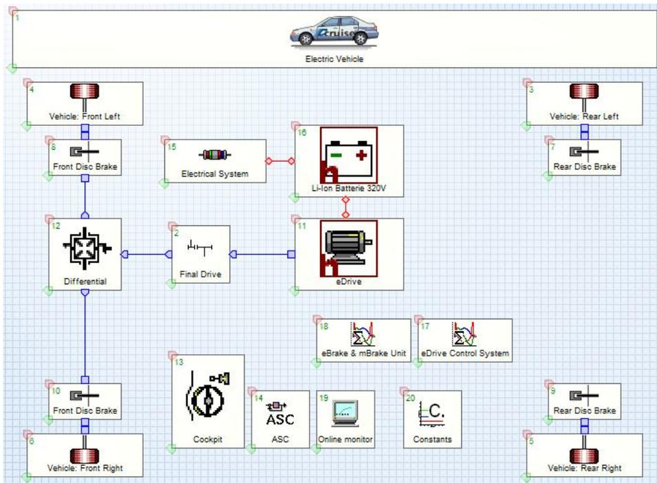
**Figure 1.** The general model of an electric vehicle with front-wheel and extension of autonomy (source AVL Cruise line 2011)
