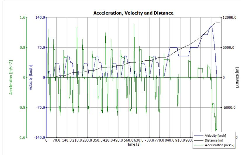
**Figure 5. Variation of acceleration, velocity and distance versus time**
