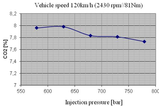
**Figure 4.** CO<sub>2</sub> emissions in percentages depending on the injection pressure for the vehicle speed of 120km/h
