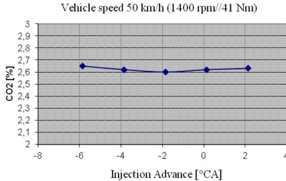
**Figure 3.** CO<sub>2</sub> emissions in percentages depending on the modification of the injection advance for the vehicle speed of 50 km/h
