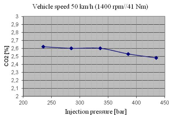
**Figure 2.** CO<sub>2</sub> emissions in percentages depending on the injection pressure
