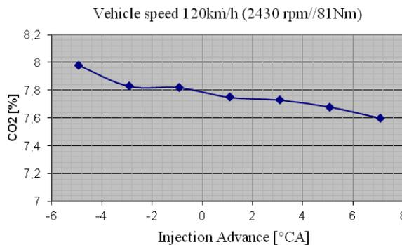
**Figure 5.** CO<sub>2</sub> emissions in percentages depending on the modification of the injection advance for the vehicle speed of 120km/h
