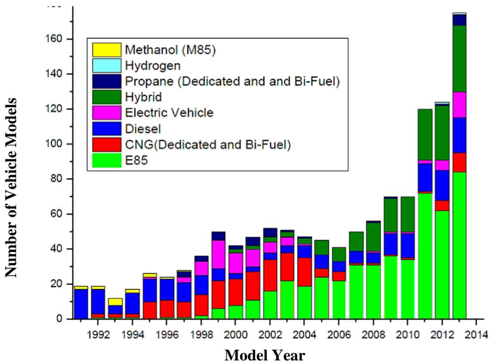
Figure 1. Number of vehicle models using different types of fuel [16]
