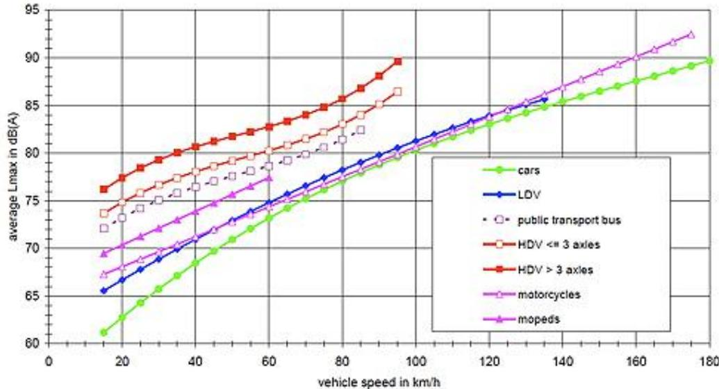
**Figure 2.** Road noise level depending on the speed and type of vehicle [16].
