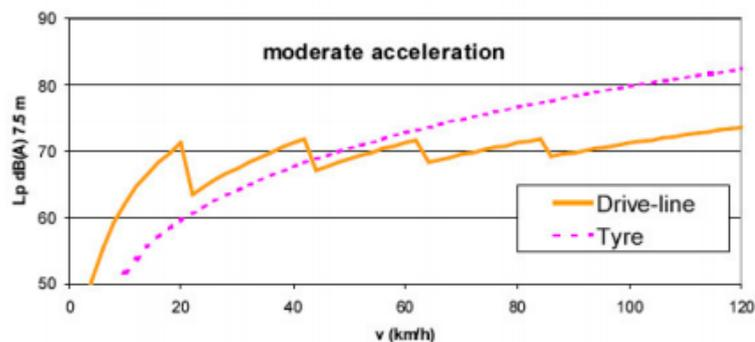
**Figure 4.** Noise level based on vehicle speed, slight acceleration [18]
