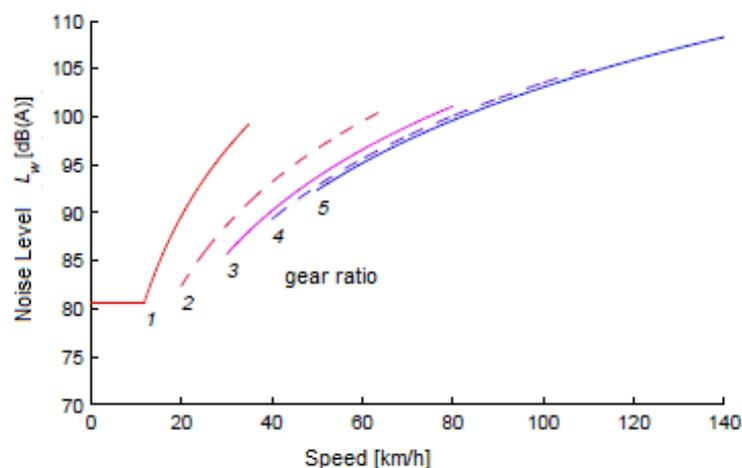
**Figure 5.** Noise level depending on gear [8]
