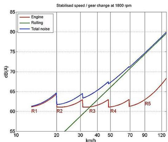
Figure 1. Road noise level depending on vehicle speed, at constant speed [15].
