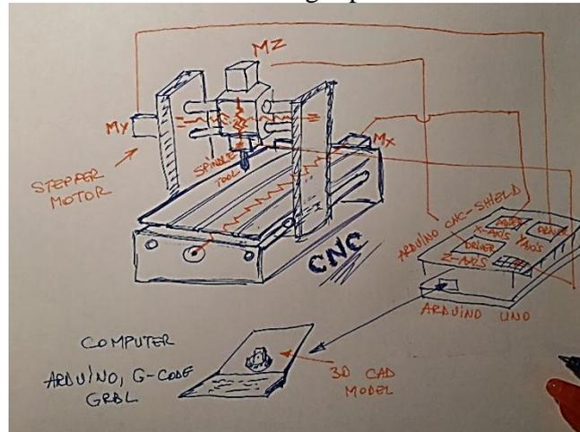
**Figure 2.** The schematic of the CNC machine concept
