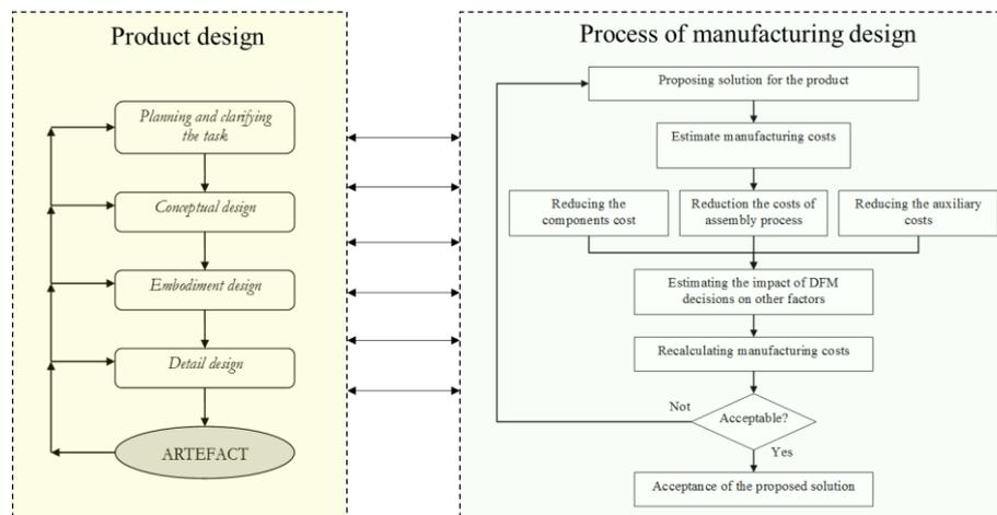
**Figure 1.** Parallel development of product/process algorithm
