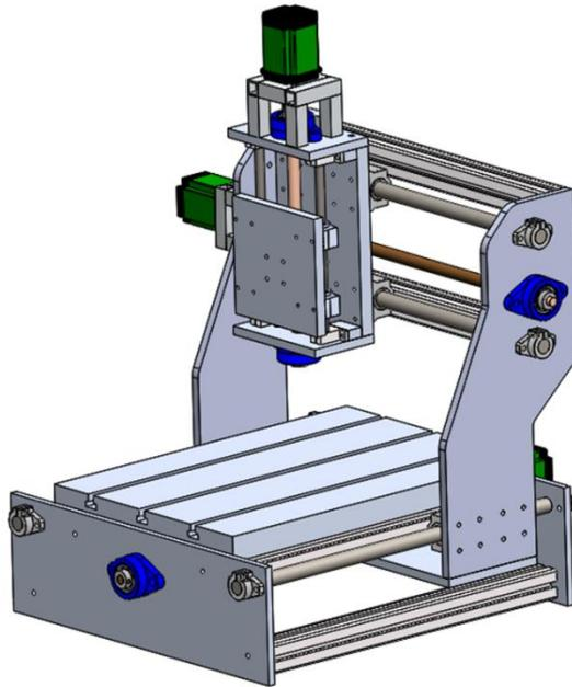
**Figure 4.** The 3D prototype of the CNC milling machine
