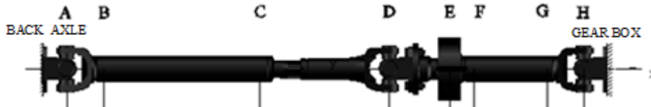
Figure 2. The Constructive model
