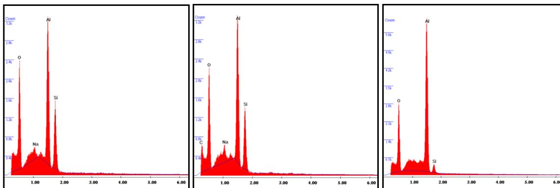
**Figure 3.** EDX spectrums of PEO oxidation film prepared at: 20, 30, 40 minutes
