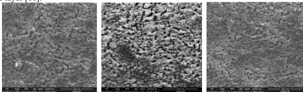
**Figure 2.** The SEM morphologies of  $\text{Al}_2\text{O}_3$  obtained at: a.20 min, b. 30 min, c. 40 mins
