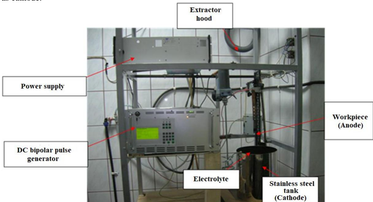
**Figure 1.** The plasma electrolytic oxidation equipment
