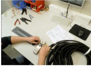
Fig. 2 Welding operation with ultrasounds
