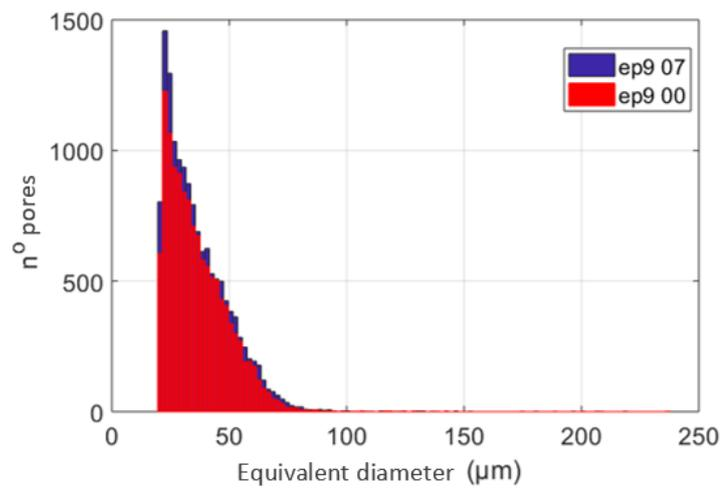
**Figure 24.** Distribution of the pores versus equivalent diameter
