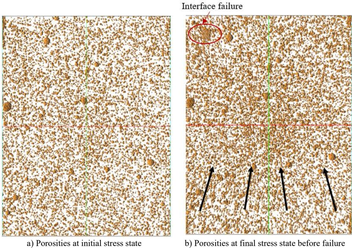
**Figure 21.** Comparison of the porosities in a slice of the adhesive joint under tensile-shear stress
