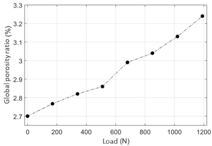
**Figure 23.** Evolution of the relative volume fraction of porosity versus load level
