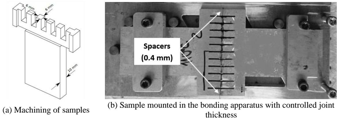
**Figure 2.** Controlled sample fixation and bonding system
