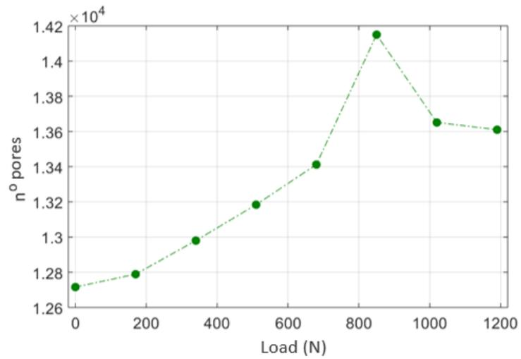
**Figure 22.** Evolution of total porosity versus load level
