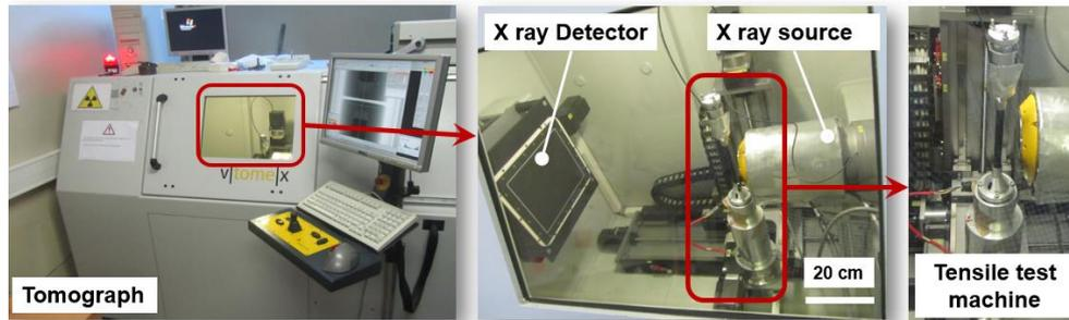
**Figure 4.** The laboratory *Phoenix VtomeX* tomograph
