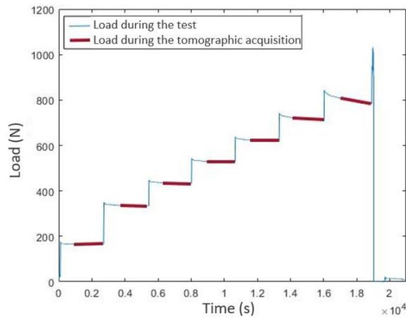
**Figure 5.** Load applied on samples
