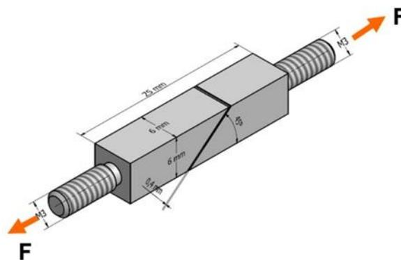
**Figure 1.** The geometry of the samples
