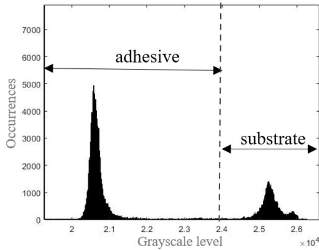
**Figure 12.** Histogram of volume and threshold calculated using the Otsu method
